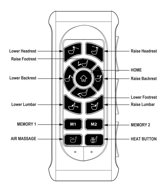
AIR MASSAGE: Press the air massage button to activate air massage function. Press again to cycle intensity through low (light is green), high (light is red), and off (light is off).
