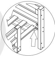
Always start assembling slat kit flush with cleat
