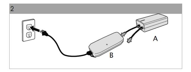
3. LED FLASHES RED when charging. SOLID GREEN LED indicates fully charged.
