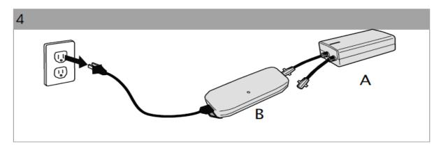
5. Then disconnect the battery pack (A) from the transformer (B)
